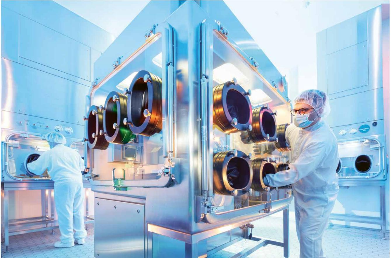
**Active pharmaceutical ingredient plant: The active ingredient tiotropium is ground in the isolator.**
